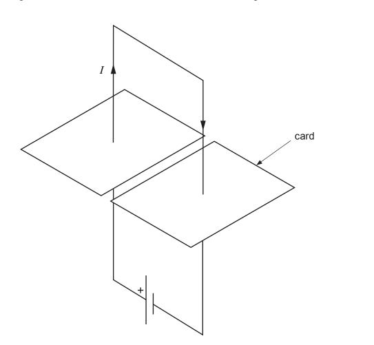
On each piece of card **draw** the magnetic field around each vertical side of the wire frame **including arrows** to show the direction of the field. [3]
